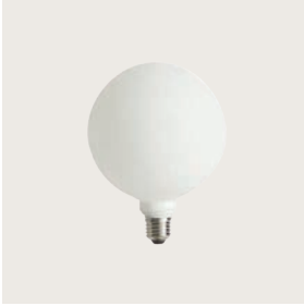
B034 140X200 E27 COB 3W 350 lm 2700K Opal Regulable / Dimmable
